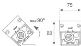
**SPÉCIFICATIONS TECHNIQUES:****Flux lumineux:** 1.386 lm**°K :** RGBW**Plum:** 57W**Efficacité:** 24,3 lm/w**Alimentación:** 110-240V 50/60Hz**Type:** MID POWER AVAGO**Équipement:** Électronique**Puissance:** 51W
