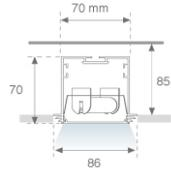
**Finish:** Shiny white RAL 9010**Dimensions:** 1.504 x 86 x 70 mm**Installation:** Recessed**Recessing measures:** 1,508 x 90 x 85 mm
