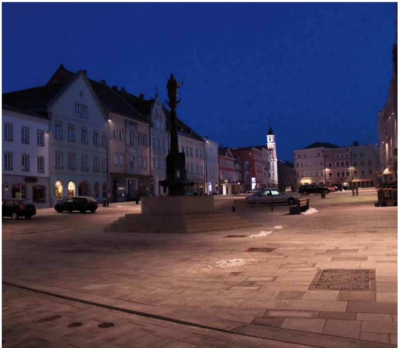
tion between the different floor zones: pedestrian area - parking area - street by variations of illuminance. Keeping the pedestrian area as free of poles as possible, the main lighting is done by façade mounted luminaires. There is only one row of poles for street lighting, which is necessary as otherwise the luminaires had to shine so low and flat that they would produce glare.
