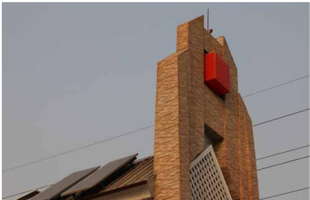
by a square aluminum frame aligned with the axis of the gate structure itself. The four low energy bulbs are also mounted on the square frame within thus achieving the absence of visible shadows on the cube when it glows.
