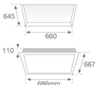
**CARACTERÍSTICAS TÉCNICAS:****Fuente de Luz:** T8/T26**Alimentación:** 230V-50HZ**Pled:** 4X18W**Equipo:** Electrónico**Casquillo:** G13
